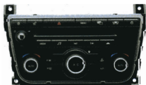
Climate Control Panel
